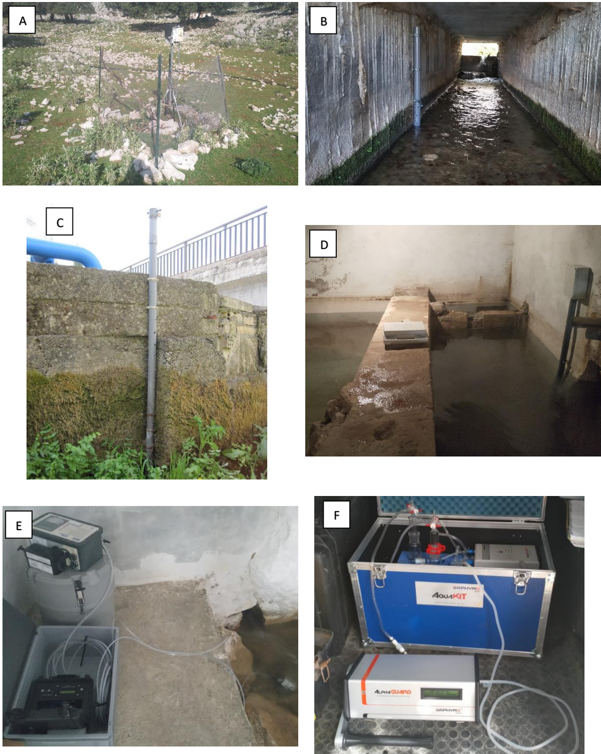
Figure 4.6: A) Weather station (WatchDog) at Sierra de Ubrique; B) Water level logger (Odyssey) at Carrizal spring; C) Water level logger (Odyssey) at Cornicabra spring; D) Conductivity meter with datalogger (WTW) installed at Carrizal spring (GW supply of Cuevas del Becerro village); E) Automatic sampler for GW collection (ISCO 3700) and field fluorometer (GGUN FL30) at Cornicabra spring (GW supply of Ubrique town) and F) Portable detector (AlphaGuard) and outgassing unit for field measurement of ^{222}\text{Rn} activity in groundwater. (Photos: Jaime Fernández Ortega and José Francisco Martín Rodríguez).
