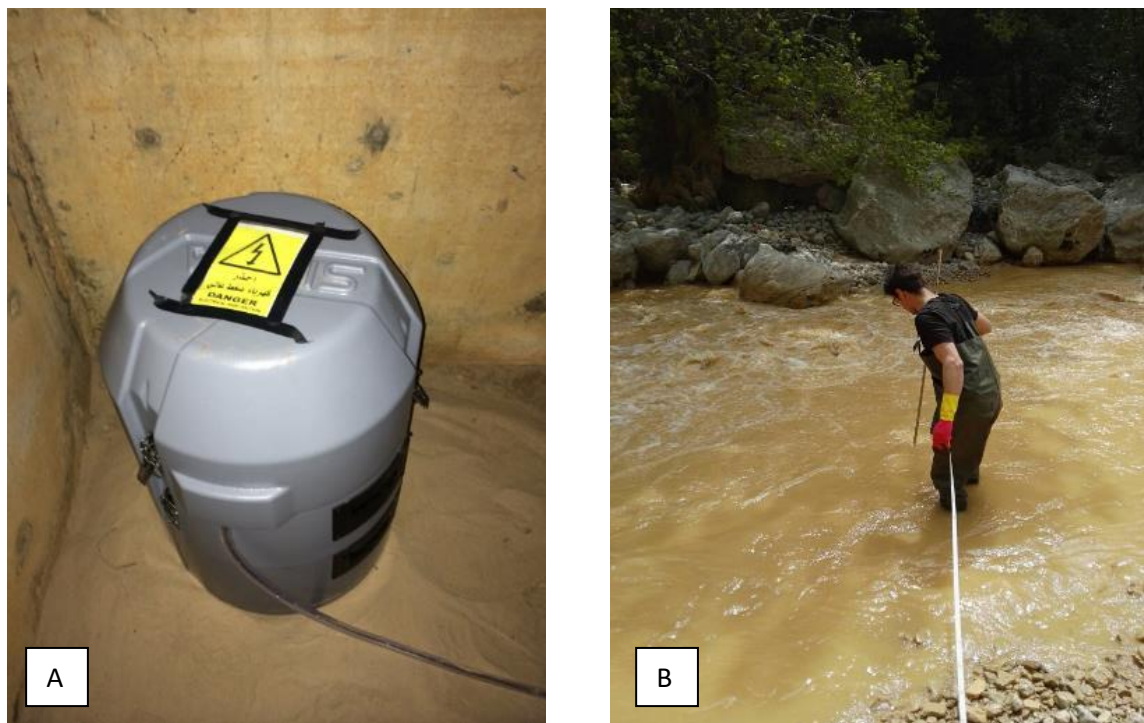
Figure 3.5: A) Automatic sampler (Sigma Hach) for water sampling every 72 hours (Photo: Joanna Doummar); B) flow measurements using a Valeport electromagnetic portable velocity meter (Photo: Michel Aoun).
