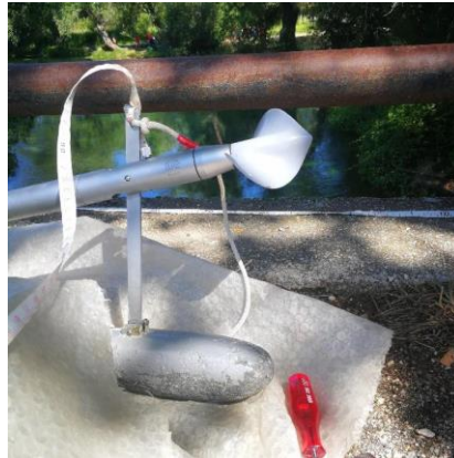
Figure 2.4: Photo of hydrometric reel for bridge measurements (Photo: Francesca Banzato).
